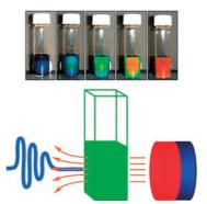
Tuning crystal: Superparamagnetic nanocrystal clusters can self-assemble into colloidal photonic crystals in solution, whose stop bands can be magnetically tuned across the entire visible spectrum. Owing to the high magnetization and the highly charged polyacrylate-capped surface of each cluster, the colloidal photonic crystals show a rapid, reversible, and widely tunable optical response to external magnetic fields.
